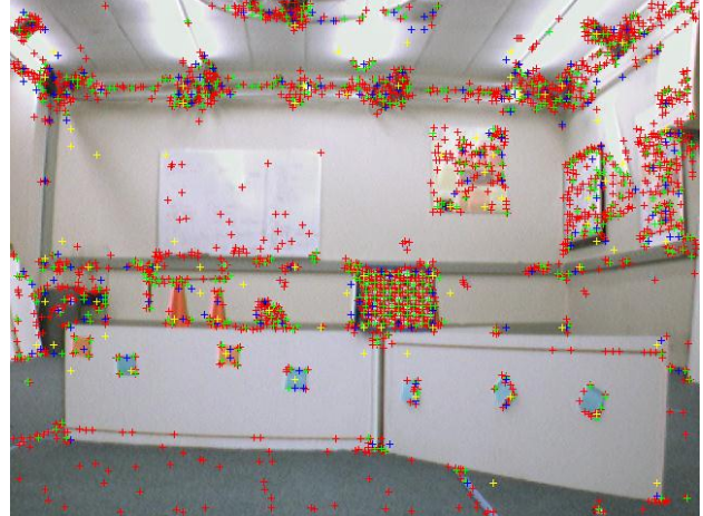
Fig 3: FAST feature extraction on a 5 level image pyramid. Different colours represent different pyramid levels. Red being the bottom level (highest resolution), followed by green, blue and yellow (lowest resolution).
